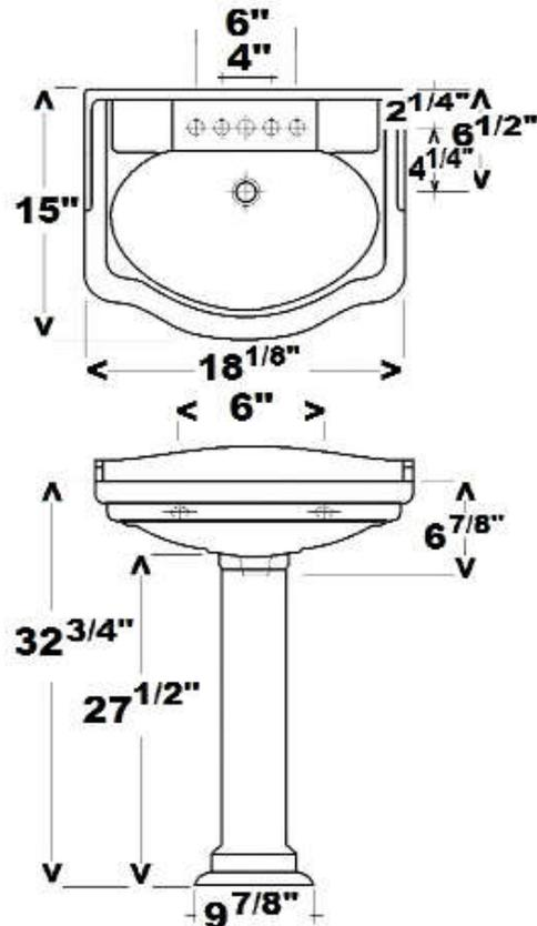
Dimensions of fixture are nominal and may vary within the range of tolerances established by ASME Standard A112.19.2-2018. Dimensions and specifications subject to change without notice.
